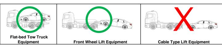
Be aware that when rolling a Honda Accord Hybrid with the front (drive) wheels on the ground, the electric motor can produce electricity and remains a potential source of electric shock even when the high-voltage system is turned off.
