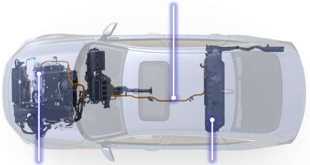
High-Voltage Air Conditioning Compressor **High-Voltage Lithium-Ion Battery**
