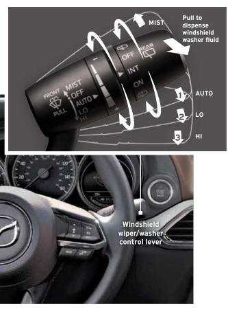
**NOTE:** Vehicles not equipped with AUTO wipers will have INT wipers. Set the lever to INT and choose an interval timing by rotating the ring between fast and slow.
