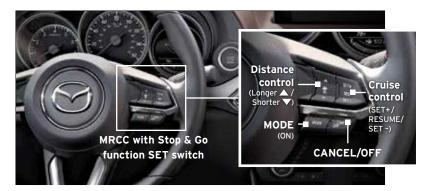
How to set the distance between vehicles: The distance between vehicles is increased by pushing the  $\blacktriangle$  switch and decreased by pushing the  $\blacktriangledown$  switch. The distance between vehicles can be set to four levels.
