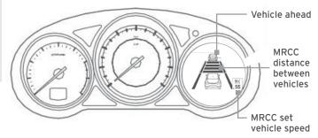
**NOTE:** The radar for the MRCC with Stop & Go function is located behind the Mazda emblem in the grille. Keep this area clean to ensure the system works properly.
