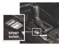
**NOTE:** If the SET button of the cruise control is pushed while in SPORT mode, SPORT mode is switched off. SPORT mode cannot be turned on or off when cornering.
