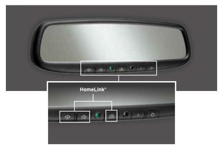
This feature provides a convenient way to replace up to three transmitters such as garage door openers, home lighting remotes and other radio frequency devices.
