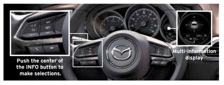
Push and hold the **INFO** button on the steering wheel to reset the currently displayed feature, such as Average MPG.
