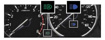
**NOTE:** When the HBC system is on, the HBC indicator light in the instrument cluster will illuminate (green). The High Beam indicator light will turn on (blue) when the HBC system switches to high beam and will turn off when the HBC system switches to low beam.
