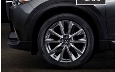
**NOTE:** Drastic changes in temperature or altitude can affect the air pressure in the tires, and may cause the TPMS warning light to turn on.
