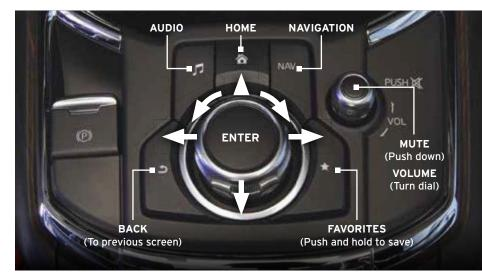
Five buttons are placed naturally beneath the fingers and mirror the on-screen icons for a more intuitive operation. Select a button around the commander switch to operate the desired function.
