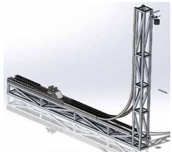
Illustration of the finalized design of the track, space frame, and launch system of the roller coaster to be constructed.
