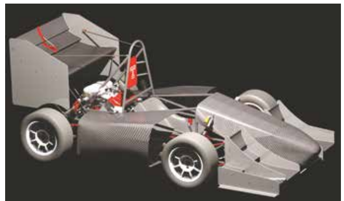
3-D rendering of the 2018 TFR car with Complete Aerodynamic Package.
