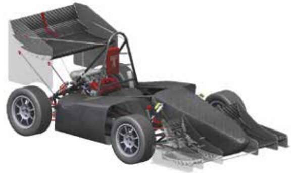
Temple Formula Racing's 2018 racecar design displaying rear wings which will be actuated with Team 52's Drag Reduction System.
