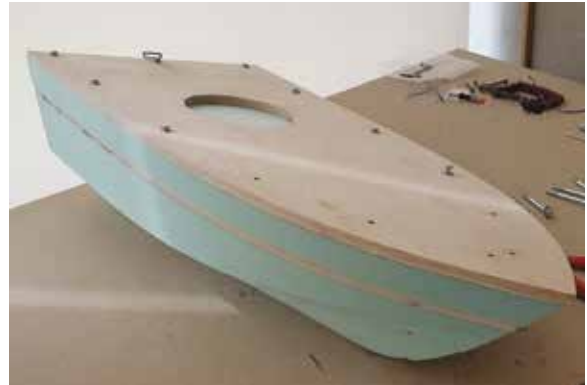
Our boat prototype, before electronics were installed and fiberglass wrapped.
