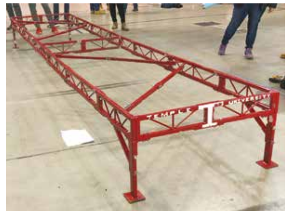
Our well built bridge, strong enough to support 2600lbs!
