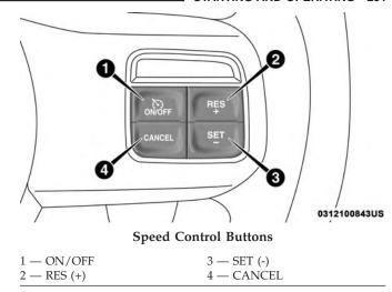
**NOTE:** In order to ensure proper operation, the Speed Control System has been designed to shut down if multiple Speed Control functions are operated at the same time. If this occurs, the Speed Control System can be reactivated by pushing the Speed Control ON/OFF button and resetting the desired vehicle set speed.
