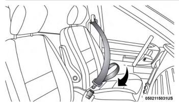
**Inserting Latch Plate Into Buckle**
