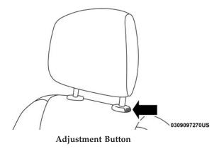
For comfort, the Active Head Restraints can be tilted forward and rearward. To tilt the head restraint closer to the back of your head, pull forward on the bottom of the head restraint. Push rearward on the bottom of the head restraint to move the head restraint away from your head.
