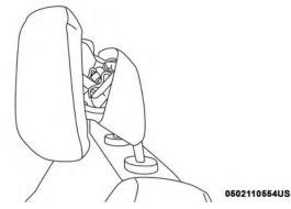
Active Head Restraint (AHR) Deployed
