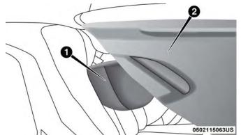
Car Seat With Head Restraint Folded
