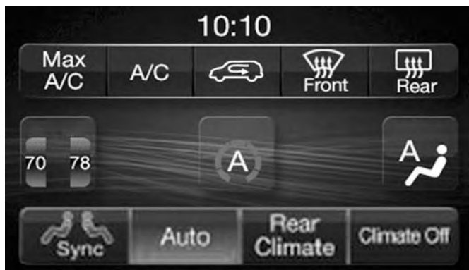
Radio 4.3 Automatic 3 Zone Temperature Controls
