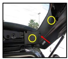
4. By hand pry the tailgate cover of the tailgate. There are 8 plastic fasteners holding the panel in place. NOTE: When removing tailgate panel continuously work around the panel and not putting too much stress in any area. (Figure B4)
