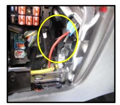
6. Install BUS Box to lower side wall with supplied double side tape. Route and plug in switch wires and OBD wires into BUS box. Connect BUS box cable to Main harness. (Figure E6a-b)
