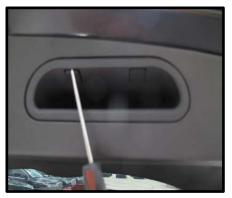
3. Place template onto rear liftgate cover with template aligned with pocket opening. Hold template in place with tape. Using the 16mm drill bit (supplied), drill at center point marked. Drill pilot hole through plastic and metal. Drill 16mm through plastic only. NOTE: it is important that you DO NOT drill through the metal with the 16mm bit, once cover is removed the hole will be drilled with 24mm bit (page 16).
