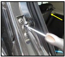
13. Using T30 Torx remove vehicle side ball mount. Using a 13mm socket, remove the upper liftgate strut ball mount from the tailgate. NOTE DO NOT replace the upper mount on the Encore. Repeat on opposite side of vehicle.
