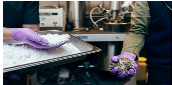
Mixed plastic waste (right) is converted to pure monomer (left) using IBM's VolCat selective digestion process.
