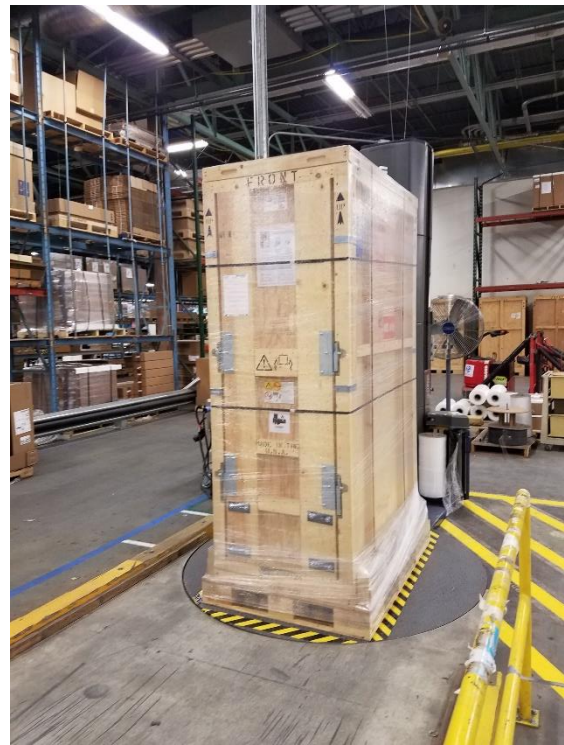
IBM z Systems® mainframe racks are shipped in reusable wooden crates. Crates are covered with a polyethylene bag to keep out rain and moisture during shipment.
