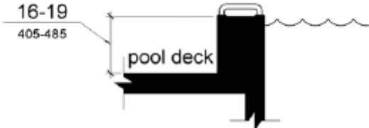
Figure 1009.4.2 Transfer Wall Height
