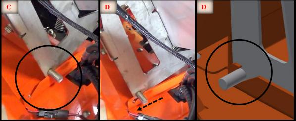
E. *Set* the **front of base** down so the Hopper Latch Rods are in the front Mounting Plate Hook.
