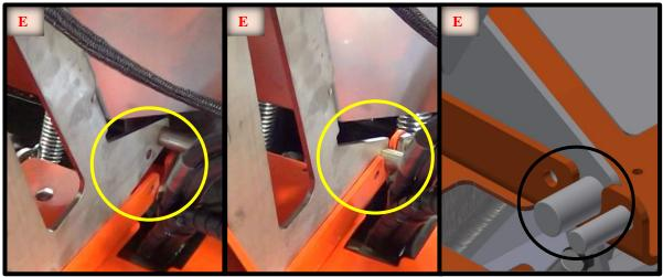
F. Attach Latches to the Hopper Latch Mounting Rods.
