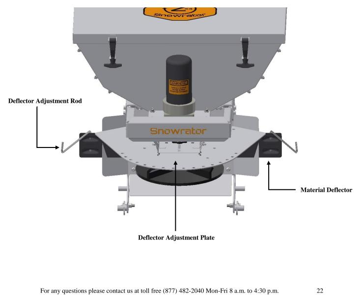
Figure 5. Directional Control Diagram
