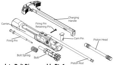
**Complete Bolt Disassembly Pt. 1**
