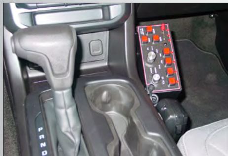
Combines siren and switch controls in one streamlined housing.
