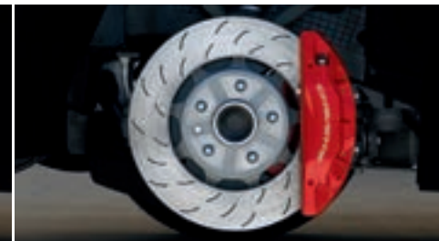
Red calipers standard on Z06 and available on Stingray, Grand Sport and ZR1 (Brembo slotted brakes included with available Z51 Performance Package shown)
