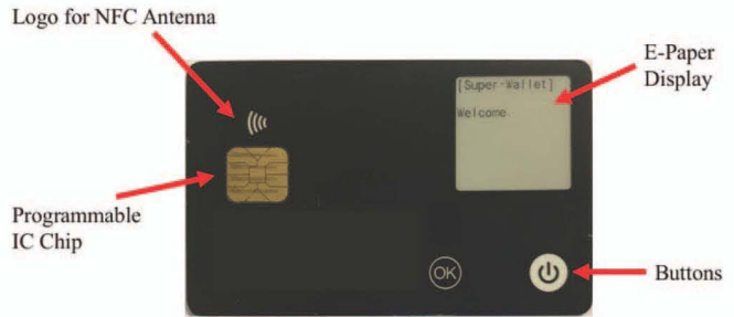
Fig. 3. Smart card with an e-paper display, physical buttons, and a programmable IC chip
