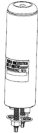
Receiver Drier (in remote condenser)
