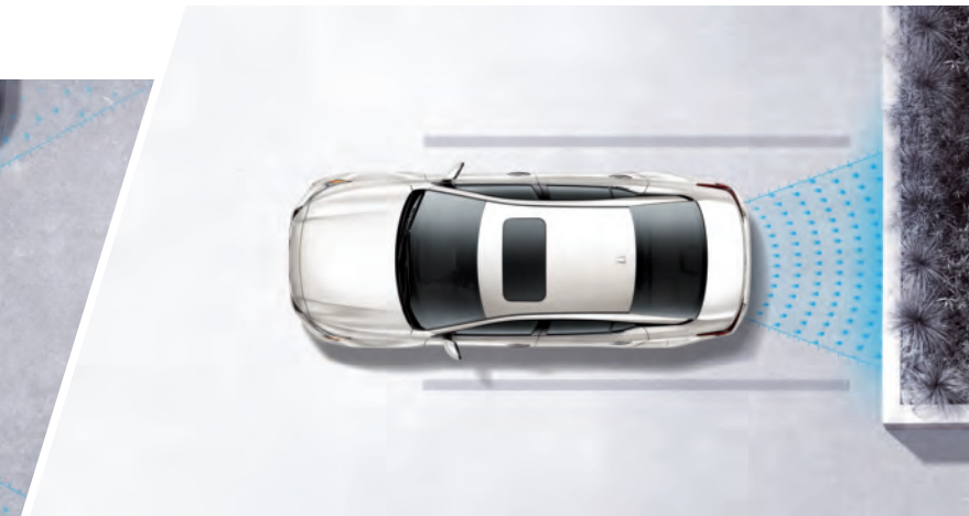
Rear Intelligent Emergency Braking Monitors the area directly behind your vehicle for stationary items you might not see. If it detects an item, and you fail to stop, it can automatically engage the brakes to help avoid a rear collision or lessen the severity of an impact. 2,10
