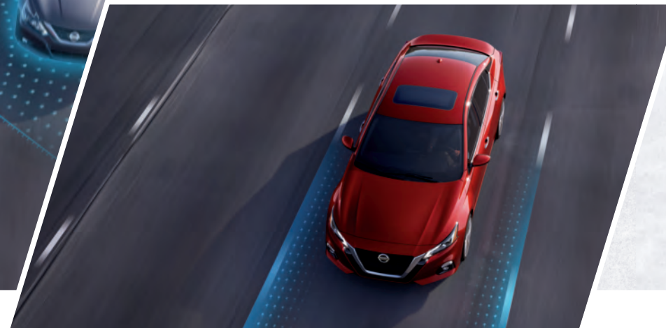
Intelligent Lane Intervention Get some help staying in your lane. When lane markings are clear, Intelligent Lane Intervention detects if you're straying out of your lane and taps the brakes to help gently guide you back. 2,6
