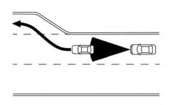
When driving on the freeway at a set speed and approaching a slower traveling vehicle ahead, the ICC system adjusts the speed to maintain the distance, selected by the driver, from the vehicle ahead. If the vehicle ahead changes lanes or exits the freeway. the ICC system accelerates and maintains the speed up to the set speed. Pay attention to the driving operation to maintain control of the vehicle as it accelerates to the set speed.
