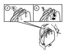
6. After closing the cap on the charge port, close the charge port lid.
