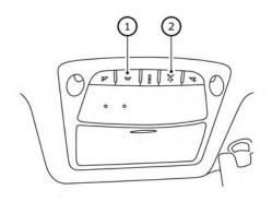
The interior lights can be turned on (1) regardless of door position. The lights will go off after a period of time unless the power switch is placed in the ON position when any door is opened.
