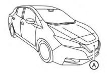
The I-FCW system uses a radar sensor (A) located on the front of the vehicle to measure distance to the vehicle ahead in the same lane.
