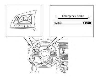
TURNING THE AFB WITH PEDESTRIAN DETECTION SYSTEM ON/OFF
