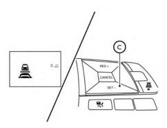
To set cruising speed, accelerate your vehicle to the desired speed, push the SETswitch © and release it. The ICC system set indicator (green), vehicle ahead detection indicator, set distance indicator and set vehicle speed indicator (B) will come on. Take your foot off the accelerator pedal. Your vehicle will maintain the set speed.
