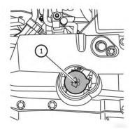
To check the fluid level, use your finger to plug the center hole (1) of the cap/tube assembly, then remove it from the reservoir. If there is no fluid in the tube, add fluid.
