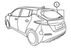
The BSW system uses radar sensors (1) installed near the rear bumper to detect other vehicles in an adjacent lane.
