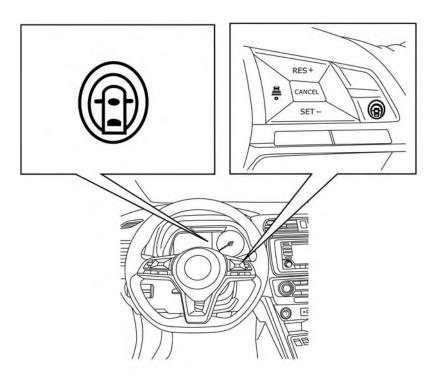
The I-LI system operates above approximately 37 mph (60 km/h). When the vehicle approaches either the left or the right side of the traveling lane, the steering wheel will vibrate and the I-LI indicator (orange) in the vehicle information display will blink to alert the driver. Then, the I-LI system will automatically apply the brakes for a short period of time to help assist the driver to return the vehicle to the center of the traveling lane.
