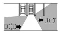
The RCTA system uses radar sensors ① installed on both sides near the rear bumper to detect an approaching vehicle.
