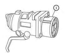
4. Align ① with the groove of the charge port and insert the charge connector.
