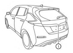
If dirt, rain or snow accumulates on the camera ①, the RearView Monitor may not display objects clearly. Clean the camera by wiping it with a cloth dampened with a diluted mild cleaning agent and then wiping it with a dry cloth.
