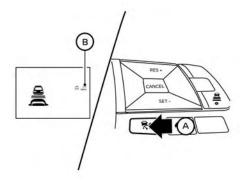
Operating vehicle-to-vehicle distance control mode
