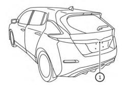
The RearView Monitor system automatically shows a rear view of the vehicle when the shift lever is shifted into the R (Reverse) position. The radio can still be heard while the RearView Monitor is active.
