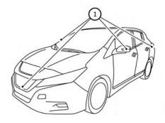
To display the multiple views, the Intelligent Around View Monitor system uses cameras located in the front grille, on the vehicle's outside mirrors and one just above the vehicle's license plate (1).
