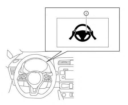
When the Steering Assist is activated, it monitors the driver's steering wheel operation.
