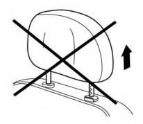
Make sure the head restraint/headrest is positioned so the lock knob is engaged in the notch before riding in that designated seating position.
