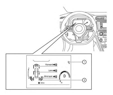
When radar blockage is detected, the system will be deactivated automatically. The BSW indicator ① will blink (yellow) in the vehicle information display. The indicator next to "Blind spot" in the "Driving Aids" menu ② will also blink (yellow).
