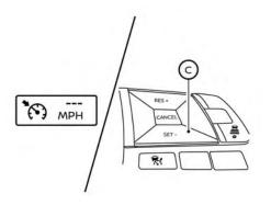
To set cruising speed, accelerate your vehicle to the desired speed, push the SET- (C) switch and release it. (The color of the cruise indicator changes to green and set vehicle speed indicator comes on.) Take your foot off the accelerator pedal. Your vehicle will maintain the set speed.
