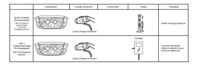
\*1: V2X (Vehicle to everything); The EV supplies electric power to a home or a building etc. (e.g. Vehicle to home (V2H), Vehicle to building (V2B), Vehicle to grid (V2G), Vehicle to load (V2L), and Vehicle to vehicle (V2V)).
