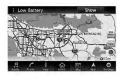
1. The notification is displayed on the upper left side of the STATUS screen. Touch [Show] to display the screen showing detailed information
