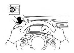
1. Take out the speed restriction sticker from the air compressor, then put it in a location where the driver can see it while driving.
