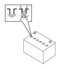
2 Check the fluid level in each cell. If it is necessary to add fluid, add only distilled water to bring the level up to the bottom of the filler opening. Do not overfill. Reinstall the vent caps.
