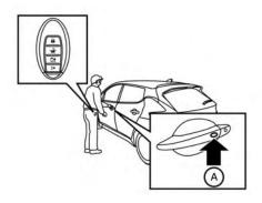
When you carry the Intelligent Key with you, you can lock or unlock all doors by pushing the door handle request switch (driver's or front passenger's) (A) or rear hatch request switch (B) within the range of operation.
