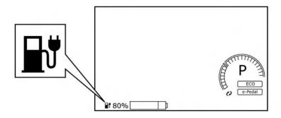
If the low battery charge indicator illuminates yellow, the Li-ion battery charge is too low for travel. For additional information, refer to "Li-ion battery available charge gauge" in the "Instruments and controls" section of this manual. Charge the Li-ion battery as soon as possible.
