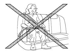
Make sure the child's head will be properly supported by the booster seat or vehicle seat. The seatback must be at or above the center of the child's ears. For example, if a low back booster seat (1) is chosen, the vehicle seatback must be at or above the center of the child's ears. If the seatback is lower than the center of the child's ears, a high back booster seat (2) should be used.
