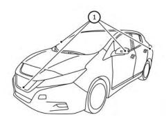
If dirt, rain or snow accumulates on any of the cameras ① , the Intelligent Around View Monitor may not display objects clearly. Clean the camera by wiping with a cloth dampened with a diluted mild cleaning agent and then wiping with a dry cloth.
