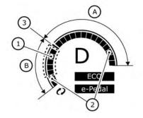
The white illuminated portion (1) moves to the left when power is generated and provided to the Li-ion battery by the regenerative brake system (Li-ion battery charging).
