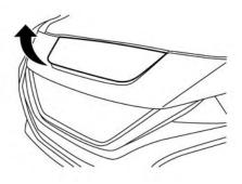
2. Put your hand into the underside of the lid and open until it is in the fully open position.
