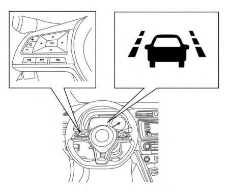
The LDW system provides a lane departure warning function when the vehicle is driven at speeds of approximately 37 mph (60 km/h) and above and the lane markings are clear. When the vehicle approaches either the left or the right side of the traveling lane, the steering wheel will vibrate and the LDW indicator in the vehicle information display will blink to alert the driver.
