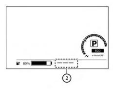
If the vehicle is driven and the Li-ion battery continues to discharge, the driving range on the instrument panel changes to "— — " ②.
