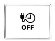
To turn off the charge timer, push the immediate charge switch. For additional information, refer to "Charging timer" in the "Charging" section of this manual.
