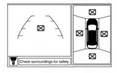
When the "[X]" icon is displayed on the screen, the camera image may be receiving temporary electronic disturbances from surrounding devices. This will not hinder normal driving operation but the system should be inspected if it occurs frequently. It is recommended that you visit a NISSAN certified I FAF dealer for this service
