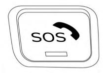
The E-call (SOS) system button is used in combination with a NissanConnect® (for Leaf) Services subscription to call for assistance in case of an emergency.
