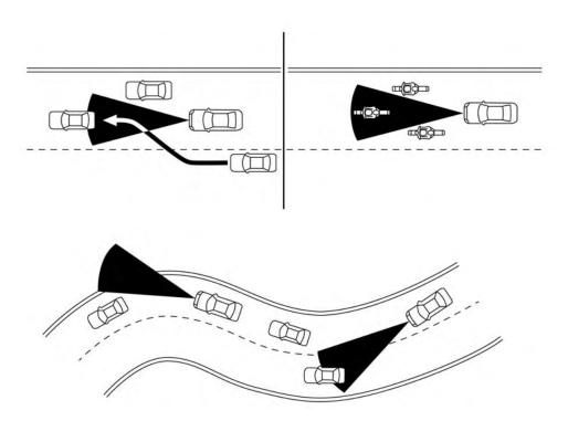
When driving on some roads, such as winding, hilly, curved, narrow roads, or roads which are under construction, the ICC sensor may detect vehicles in a different lane, or may temporarily not detect a vehicle traveling ahead. This may cause the ICC system to decelerate or accelerate the vehicle.
