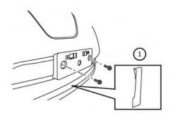
To mount the front license plate, attach the license plate bracket 10 to the bumper fascia at the location marks (small dimples) using the two provided screws.
