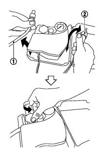
2. Take the hose 1 and the power plug 2 out of the air compressor. Remove the cap of the bottle holder from the air compressor.
