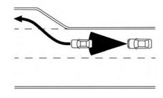
When driving on the freeway at a set speed and approaching a slower traveling vehicle ahead, the ICC system will adjust the speed to maintain the distance, selected by the driver, from the vehicle ahead. If the vehicle ahead changes lanes or exits the freeway, the ICC system will accelerate and maintain the speed up to the set speed. Pay attention to the driving operation to maintain control of the vehicle as it accelerates to the set speed.
