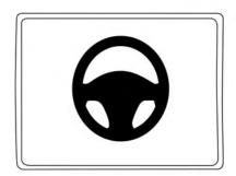
The Steering Assist switch is used to enable and disable the Steering Assist system that is activated using the settings menu of the vehicle information display.
