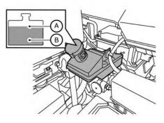
Check the fluid level in the reservoir If the fluid is below the MIN line (B) or the brake warning light illuminates, add Genuine NISSAN Super Heavy Duty Brake Fluid or equivalent **DOT 3** fluid up to the MAX line (A). If fluid must be added frequently, the system should be checked. It is recommended that you visit a NISSAN certified LEAF dealer for this service
