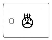
The heated steering wheel system is designed to operate only when the surface temperature of the steering wheel is below approximately 68°F (20°C).
