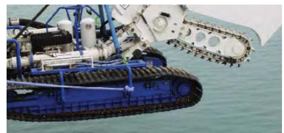
Subsea Trench Cutting Machinery (Source: Louis Dreyfus Travocean)
