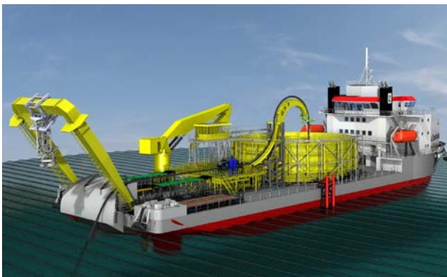
New Generation of Cable Laying Vessel—Courtesy Boskalis
