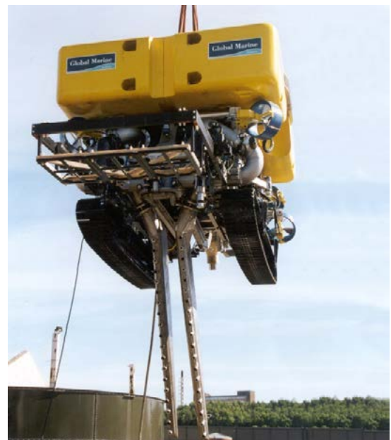
Typical Tracked-ROV Jetting Machine (Source: Global Marine)
