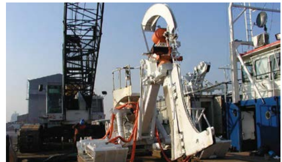
Subsea Vibrating Plough (Source: Louis Dreyfus Travocean)
