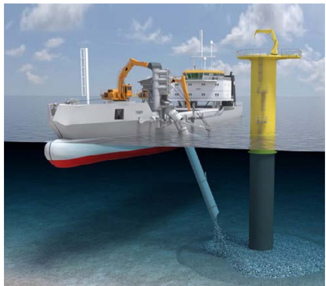
Rock Dump Vessel—Side Stone Dumping Systems and Flexible Fall Pipe System (Source: IADC and Seahorse)
