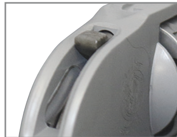
Shrouded Hammer for Easy Holstering while allowing for Single Action Fire
