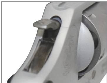
External Hammer for Single Action Fire
