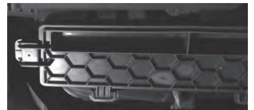
Cover to air filter housing is now exposed and can be removed.
