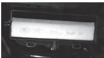
Remove cabin air filter.
