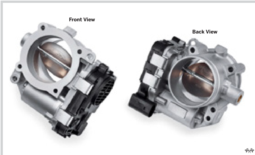
C. SCREAMIN' EAGLE PRO HIGH-FLOW 64MM EFI THROTTLE BODY – ELECTRONIC THROTTLE
