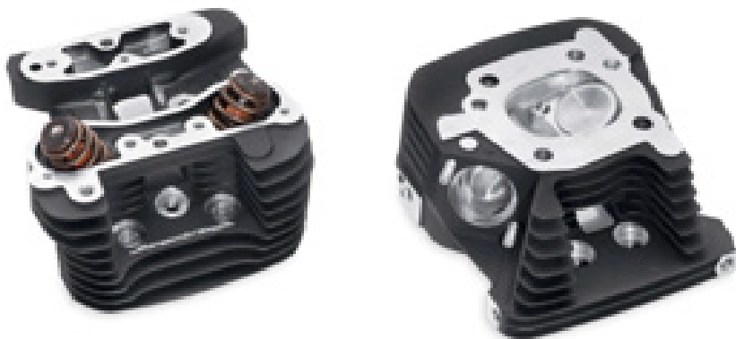
C. SCREAMIN' EAGLE PRO CNC PORTED FACTORY CYLINDER HEADS – SPORTSTER (16500074 SHOWN)
