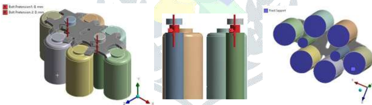
Figure 6: Boundary conditions and meshing (bolt pretension and fixed support)
