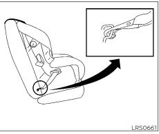
LATCH webbing-mounted attachment Installing child restraint LATCH lower anchor attachments
