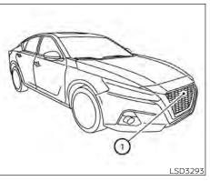
The I-FCW system uses a radar sensor () located on the front of the vehicle to measure the distance to the vehicle ahead in the same lane.
