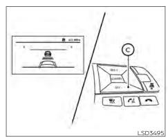
To set cruising speed, accelerate your vehicle to the desired speed, push the SETswitch and release it. The ICC system set indicator (green), vehicle ahead detection indicator, set distance indicator and set vehicle speed indicator (a) will come on. Take your foot off the accelerator pedal. Your vehicle will maintain the set speed.
