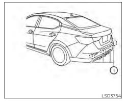
Do not attach stickers (including transparent material), install accessories or apply additional paint near the sonar sensors.
