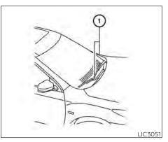
Be sure you do not put anything on top of the autolight sensor located in the top side ① of the instrument panel. The autolight sensor controls the autolight; if it is covered, the autolight sensor reacts as if it is dark out and the headlights will illuminate. If this occurs while parked with the engine off and the ignition switch placed in the ON position, your vehicle's battery could become discharged.
