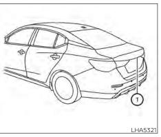
To display the rear view, the RearView Monitor system uses a camera located just above the vehicle's license plate  $\bigcirc$ .
