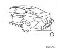
The RAB system detects obstacles behind the vehicle using the parking sensors  $\bigcirc$  located on the rear bumper.
