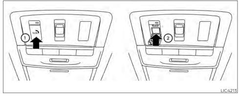
The E-call (SOS) button is used in combination with a NissanConnect® Services subscription to call for assistance in case of an emergency.
