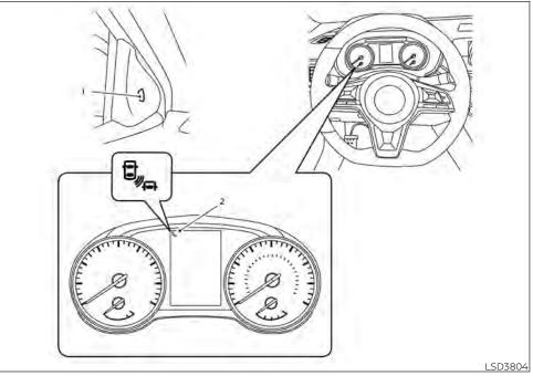
The RCTA system can help alert the driver of an approaching vehicle when the driver is backing out of a parking space.
