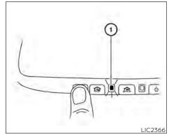
Using both hands, simultaneously press and hold the desired HomeLink® button and hand-held transmitter button. DO NOT release until the HomeLink® indicator light ① flashes slowly and then rapidly. When the indicator light flashes rapidly, both buttons may be released. (The rapid flashing indicates successful programming.)
