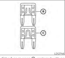
5. If the fuse is open B, replace it with an equivalent good fuse  $\bigodot{}$ .
