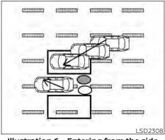
**Illustration 6 – Entering from the side Illustration 6:** If the driver activates the turn signal while another vehicle is in the detection zone, then the system chimes (twice) and the side BSW/RCTA indicator light flashes.
