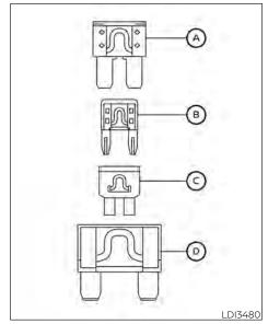
Four types of fuses are used. Type  $\textcircled{\mbox{\sc op}}$  is used exclusively in the passenger compartment fuse box.
