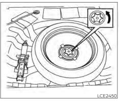
4. Turn the clamp counterclockwise and remove to release the spare tire.
