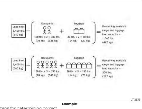
Steps for determining correct load limit
