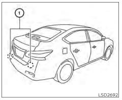
The BSW system uses radar sensors installed near the rear bumper to detect other vehicles in an adjacent lane.
