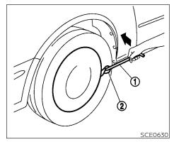
Removing wheel cover (if so equipped)
