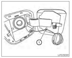
To remove the fuel-filler cap:
