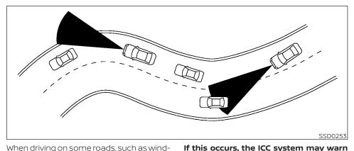
When driving on some roads, such as winding, hilly, curved, narrow roads, or roads which are under construction, the ICC sensor may detect vehicles in a different lane, or may temporarily not detect a vehicle traveling ahead. This may cause the ICC system to decelerate or accelerate the vehicle.
