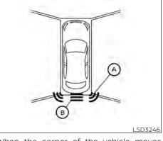
When the corner of the vehicle moves closer to an object, the corner sonar indicator O appears. When the center of the vehicle moves close to an object, the center sonar indicator B appears.
