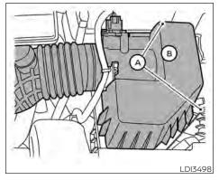
The viscous paper type filter element (if so equipped) should not be cleaned and reused. The dry paper type filter element (if so equipped) may be cleaned an reused. Replace it according to the maintenance log shown in the "Maintenance and schedules" section of this manual.
