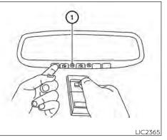
Position the end of your hand-held transmitter 1-3 in (2-8 cm) away from the HomeLink<sup>®</sup> surface, keeping the HomeLink<sup>®</sup> indicator light () in view.
