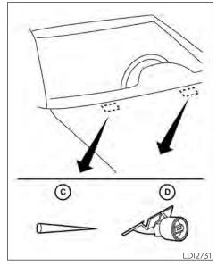
If you wax the surface of the hood, be careful not to let wax get into the washer nozzle 0. This may cause clogging or improper windshield-washer operation. If wax gets into the nozzle, remove it with a needle or small pin 0.
