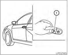
If a door handle is pulled while unlocking the doors, that door may not be unlocked. Returning the door handle to its original position will unlock the door. If the door does not unlock after returning the door handle, push the door handle request switch (if so equipped) to unlock the door.
