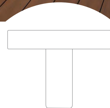
BUILDER RAIL TOP RAIL SIZE: 3.4" X 1.5"
