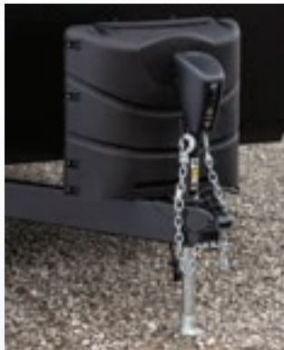
(2) 20 Lb. LP bottles with cover, manual jack with chain hooks – standard. (Power Stance tongue jack and auxiliary cord – optional)
