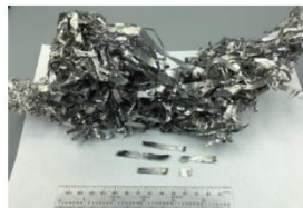
Perfect Fe – 6.5 wt.% Si produced by large melt spinner
