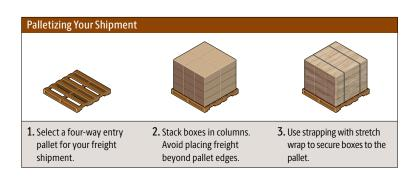
Pallets with four-way forklift entry are preferred as they help to improve handling and reduce damage to the shipment
