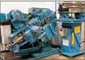
WATERBURY FARREL #30 incline thread roller
