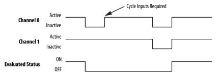
If inputs are configured with the following dual channel settings, an Input fault occurs if the inputs are discrepant for longer than 3 seconds or if a 'cycle inputs required' condition exists lor longer than 3 seconds.
