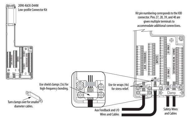
Refer to the Kinetix 6200 and Kinetix 6500 Modular Multi-axis Servo Drive User Manual, publication <u>2094-UM002</u>, for safety, auxiliary feedback, and I/O signal descriptions and wiring examples when using the 2090-K6CK-D44M connector kit.
