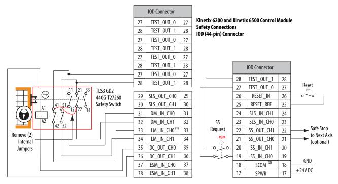
(1) Lock monitoring connections are not required for Safe Limited Speed with Door Monitoring mode operation.
