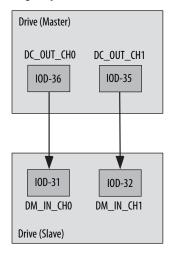
Only the wiring configurations shown below are supported for the Door Control output.
