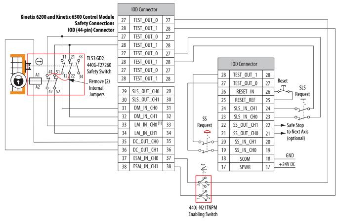
(1) Lock monitoring connections are not required for Safe Limited Speed with Door Monitoring and Enabling Switch Monitoring mode operation.
