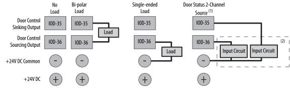
When wired as a source for a safety input, current is limited to 20 mA per output. (1) (2)
