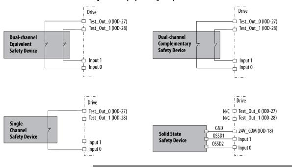
Figure 4 - Safety Input Wiring Examples
