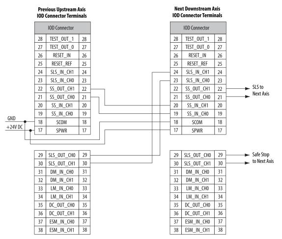
This second example is configured as a cascaded last unit via the [System Configuration] parameter. It has SS\_In, SLS\_In, and DM\_In input connections from the previous upstream drive, but its SS\_Out, SLS\_Out, and DC\_out outputs are connected to a Bulletin 1791DS module.
