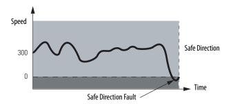
Figure 46 - Negative Safe Direction Monitoring Timing Diagram
