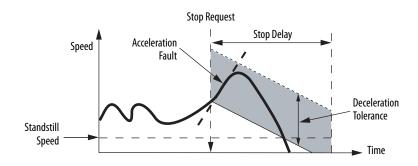
If an Acceleration fault is detected during the Stop Delay [Maximum Stop Time] and the [Safe Maximum Acceleration Monitoring Stop Behavior] parameter equals Use Safe Torque Off with Check for Standstill, the Acceleration fault is reported and Motion Power is removed. The Stop Delay [Maximum Stop Time] continues with standstill checking enabled.
