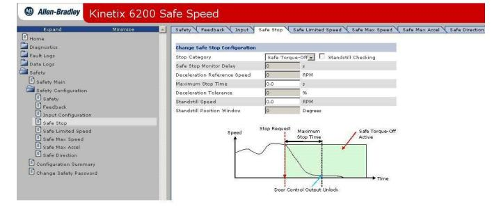
3. From the Stop Category pull-down menu, choose Safe Torque-Off (default) and check the Standstill Checking box, as the parameter value.
