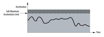
You define the Stop Category initiated by the drive in the event of an Acceleration fault by using the [Safe Maximum Acceleration Monitoring Stop Behavior] parameter.
