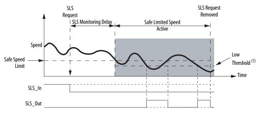
(1) Low Threshold = (Speed Hysteresis/100) x Safe Speed Limit
