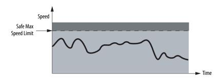
You define the Stop Category initiated by the drive in the event of an SMS Speed fault by using the [Safe Maximum Speed Monitoring Stop Behavior] parameter.
