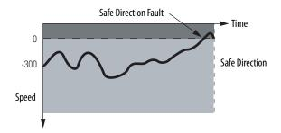
If motion is detected in the incorrect direction while Safe Direction Monitoring is active, a Direction fault occurs. If a Direction fault is detected while the drive is monitoring motion, the configured [Stop Category] is initiated and direction monitoring is not performed during the safe stop. If a Direction fault is first detected after the initiation of the safe stop, then all outputs go to their faulted state.
