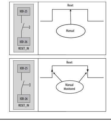
**IMPORTANT** If you configure the drive for automatic reset, wiring of the reset input terminal (IOD-26) is not required.
