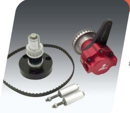
Includes the new Aeromotive Belt Drive Fuel Pump P/N 11105, and all the components necessary for mounting. This kit comes with drive mandrel, pump pulley, crank shaft pulley, cog belt, universal mounting bracket, adjustment shims and hardware. Please call, fax or e-mail for information on proper kits to match your application.
