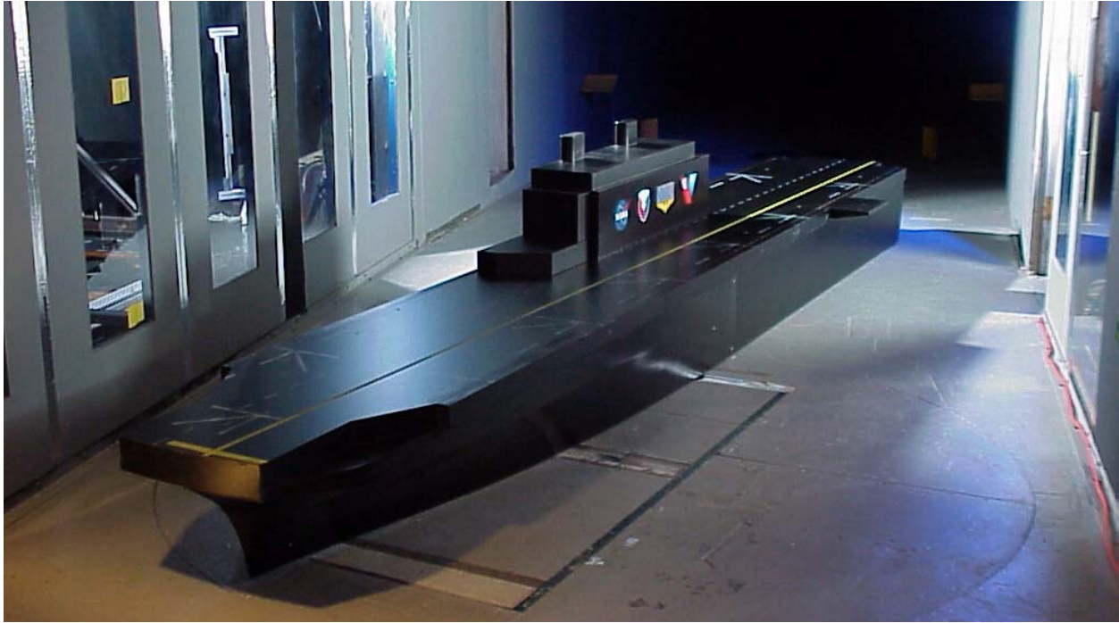
Figure 1. 1/48 th -scale amphibious assault ship installed in Army 7- by 10-Foot Wind Tunnel at NASA Ames.
