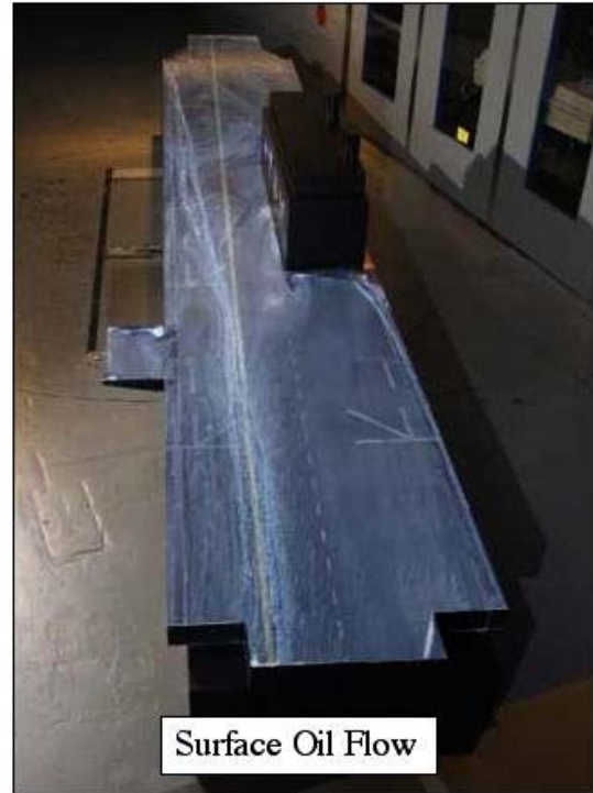
Figure 5. Surface oil flow visualization of deck for yaw = 15 deg. View from rear of ship.
