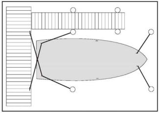
Securing The Boat In A Slip (Typical)
