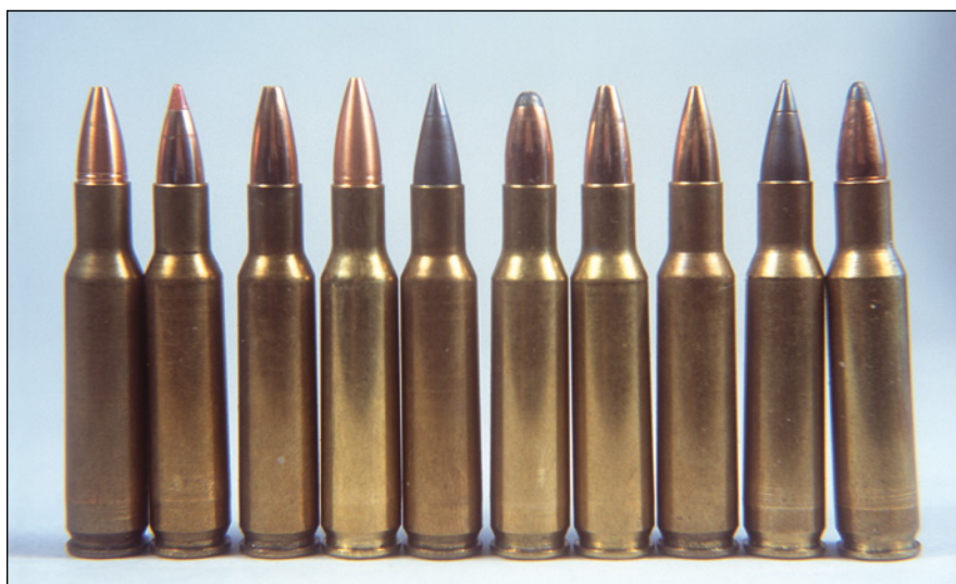
Sample bullets loaded for testing include, from left: Cutting Edge 32-grain PHD, Nosler 35 Lead Free, Berger 40 HP, Cutting Edge 40 FB, Hornady 40 V-MAX, Nosler 45 SB, Barnes 50 Varminator, Berger 50, Hornady 50 V-MAX and Hornady 55 Spire Point.
