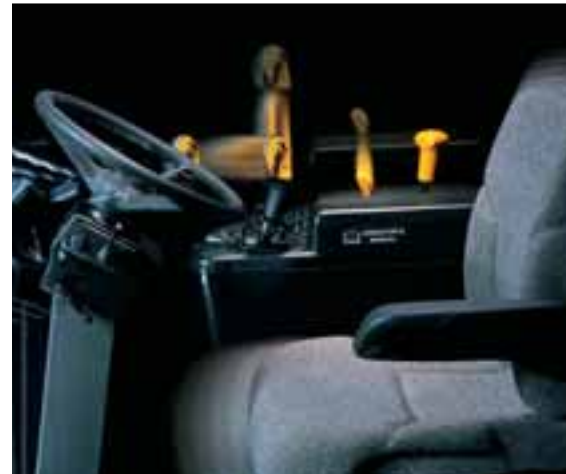
The right-hand console adjusts to fit any operator. In addition, the steering column pivots both at the wheel and at the floor.
