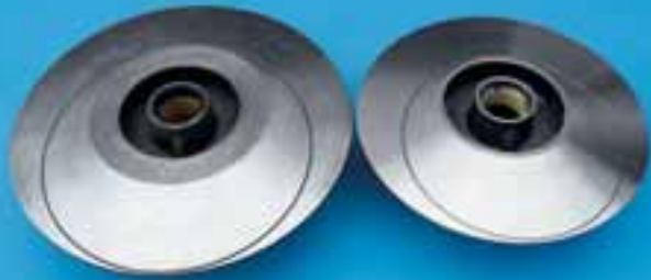
Larger-diameter rotor pulley Previous rotor pulley
