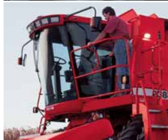
New delayed exit lighting will remain illuminated for 30 seconds after the field lighting switch is turned off for improved night-time exit.
