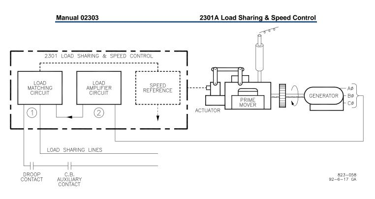
Figure 4-3. Paralleling System
