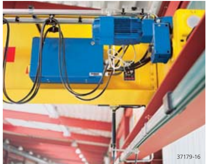
A crane end truck driven by an offset gear motor
