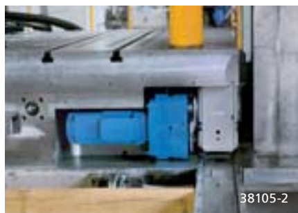
A cylindrical-rotor brake motor moves a tool-changing carriage into the exactly specified positions
