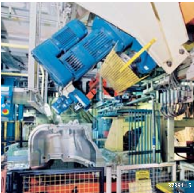
Drive for starting and stopping applications with short cycle times and high positioning accuracy in an automotive welding line
