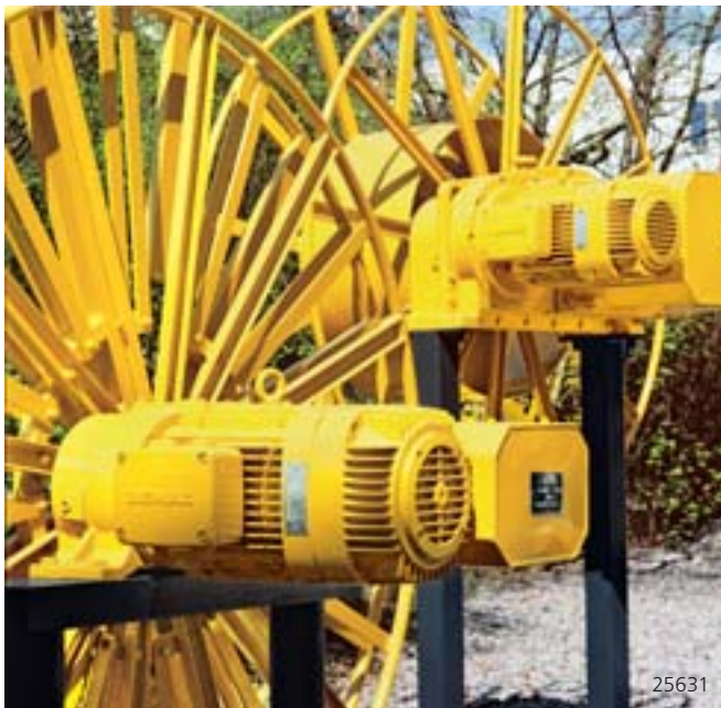
A cable drum driven by a KBS motor
