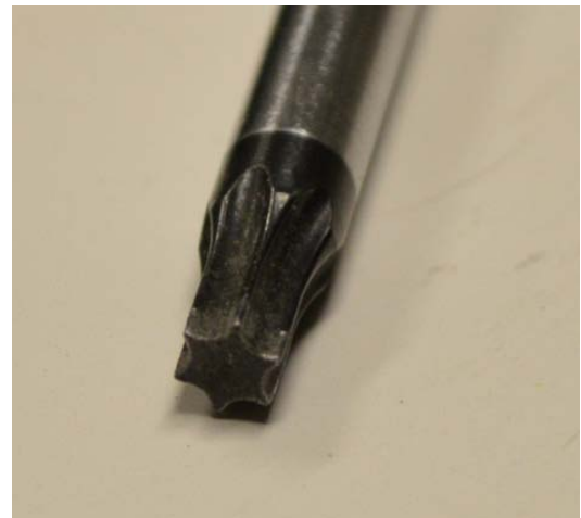
"TORX" T20 DRIVER FOR OPENING CONTROL-BOX
