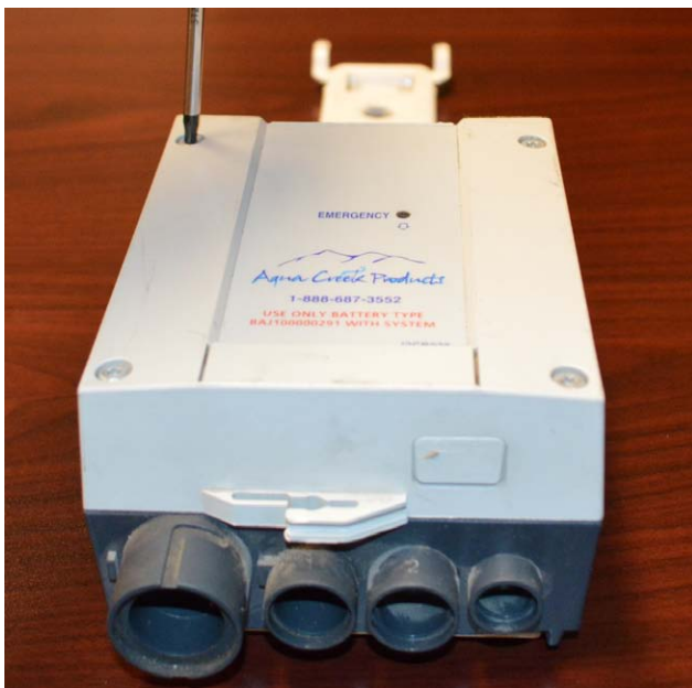
REMOVE THE FOUR (4) SCREWS FROM THE TOP OF THE CONTROL BOX: LEAVE SCREWS IN HOLES
