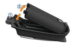
3 Insert four AA batteries, observing polarity.
