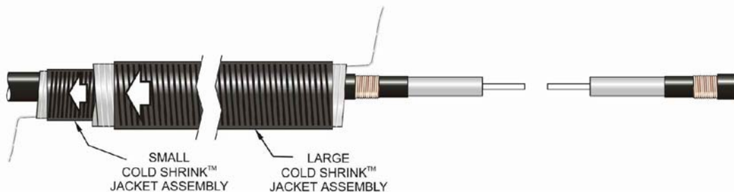
FIGURE 2 PLACING COLD-SHRINK JACKET ONTO CABLE
