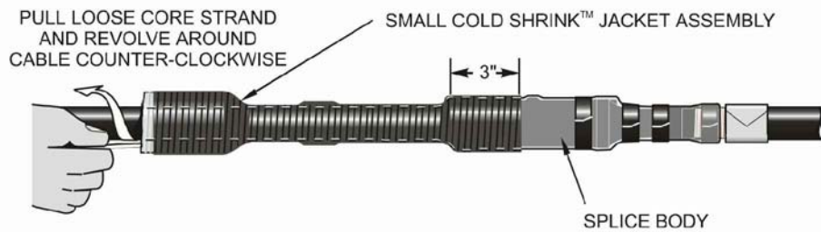
FIGURE 11 INSTALLING SMALL COLD-SHRINK JACKET ASSEMBLY
