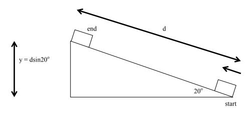
We will compare the starting point at the bottom of the ramp (where we will define  $U_g = 0$ ) and the ending point at the highest point reached by the sled. So, kinetic energy at the bottom gets converted into gravitational potential energy at the top, as well as thermal energy produced by the non-conservative friction force.
