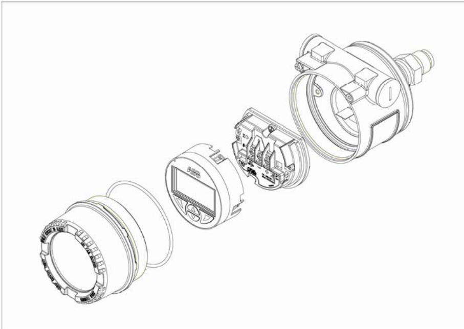
Transmitter Sectional View for the 364 models with Digital LCD Integral Display
