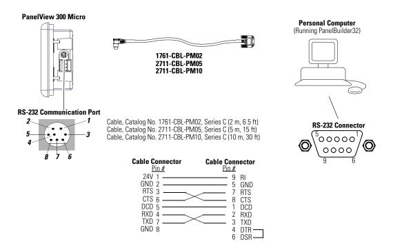
Refer to the PanelBuilder32 software user manual for application download instructions. Here's a short summary of the methods that can be used to transfer files to a PanelView 300 Micro terminal.
