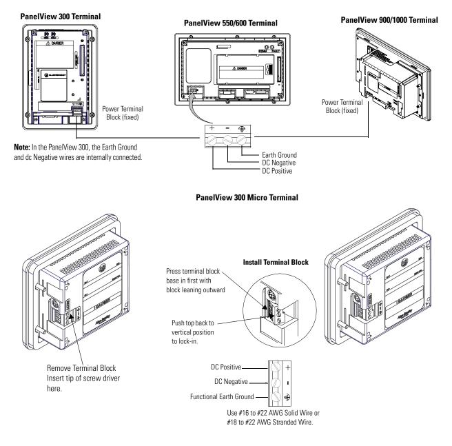
**2.** Secure the Functional Earth Ground (FE) wire to the correct terminal block screw.
