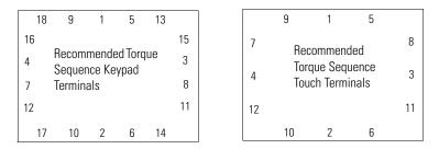
Note the sequence starts at center studs and continues to the corner studs.
