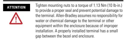
**8.** Alternately tighten the self-locking nuts (use 3/8 in. socket) until the PV1400 terminal is held firmly against the panel.
