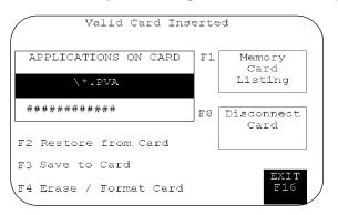
If necessary, press Erase/Format Card, [F4] key on keypad terminals, to format or erase a 2711-NM11, 2711-NM12, 2711-NM13, 2711-NM14, or 2711-NM15 memory card.
