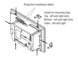
**6.** Alternately tighten the mounting clip screws to a torque of 1.13 Nm (10 lb-in).
