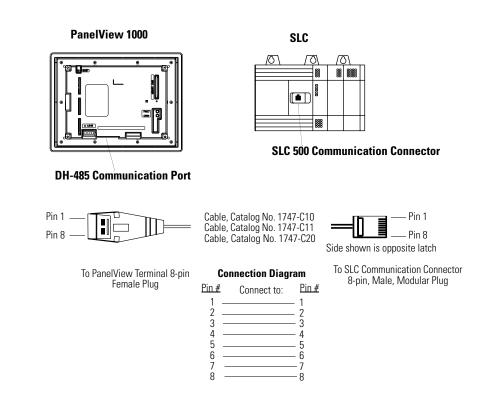
The DH-485 connectors are not electrically isolated. If electrical isolation is required, use Link Couplers (Cat. No. 1747-AIC) as shown on next page.
