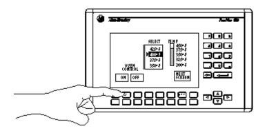
A function key legend kit is available for each terminal (except the PV300 Micro terminal) to create custom labels for the function keys.
