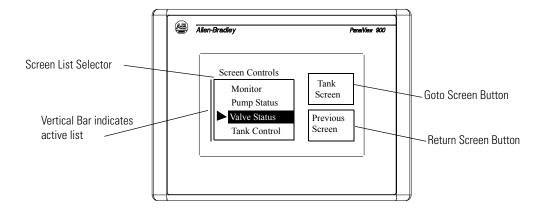
Goto and Return screen buttons can have a variety of appearances such as unique inner text, fill pattern, border or shape. Return screen buttons display the previous screen. Goto screen buttons display the assigned screen.
