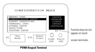
Note: On PV550/600 terminals, the Reset Video is F9. On PV300 and PV300 Micro terminals, the Reset Video is F2.
