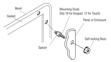
**5.** Make sure the sealing gasket is properly positioned on the terminal.
