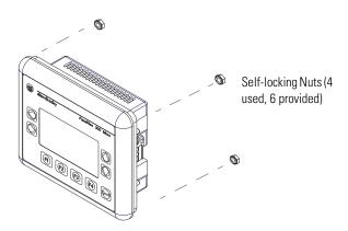
**5.** Alternately tighten the self-locking nuts until the terminal is held firmly against the panel.
