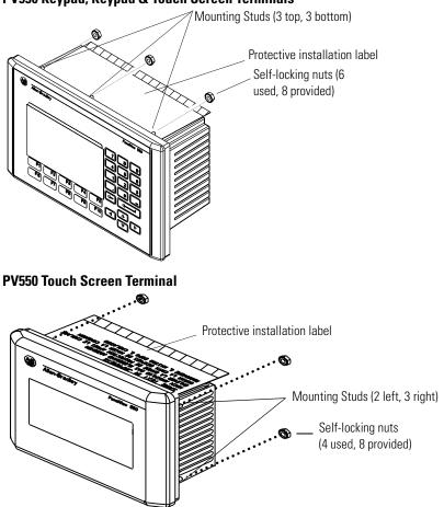
PV550 Keypad, Keypad & Touch Screen Terminals
