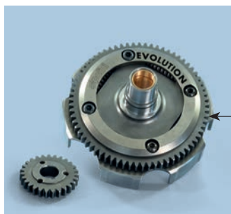
202.1221 Vespa 50 Z=24/72 Primary ratio-Primario
