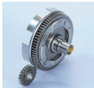
202.1216 Vespa 50 75/90 Z=24/72 Primary ratio-Primario
