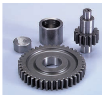
202.1321 Mbk Booster-Aprilia Z=14/41 Secondary ratio-Secondario
