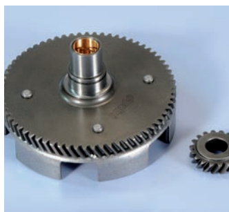
202.1218 Vespa 50/75 Z=18/67 Primary ratio-Primario
