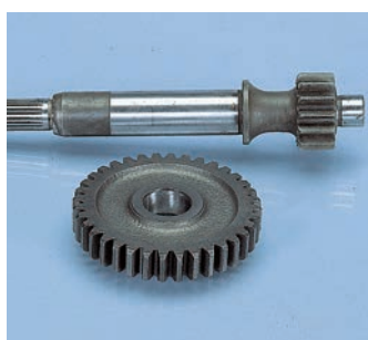
202.1334 Cagiva City Z=17/41 Primary ratio-Primario
