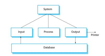
**Figure 28.1** An input-processoutput model of a data processing system
