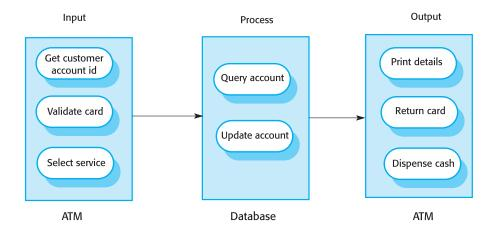
Figure 28.4 The software architecture of an ATM
