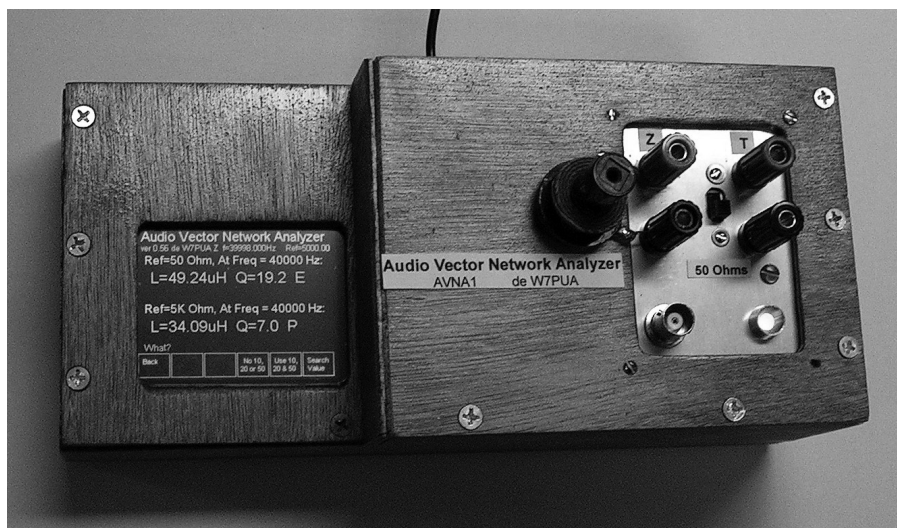
Figure 12 — The AVNA screen shows the result of using the “What?” function to determine the best measurement of a Pi inductor marked as 50 \mu\text{H} , using the 50 \Omega and 5 k \Omega reference resistors. The quality grade is shown on the right edge, with “E” meaning excellent, and “P” for poor. The value of this inductor allows it to have excellent quality with 50 \Omega and at 40 kHz. Other quality grades are “G” for good and “O” for don’t use.
