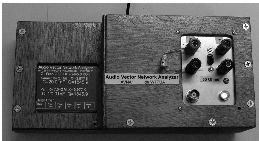
Figure 7 — The AVNA shows the measurement of a 20 nF capacitor at 2,000 Hz.
