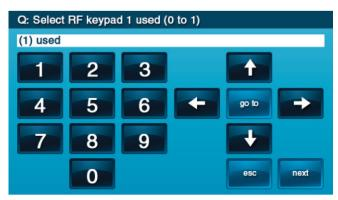
Set the RF Keypad Equipment Code to 1059 by pressing the → arrow until "(1059) 2GIG-TS1 wireless touchscreen keypad" appears. Press the  $\downarrow$  arrow to advance to the next option.
