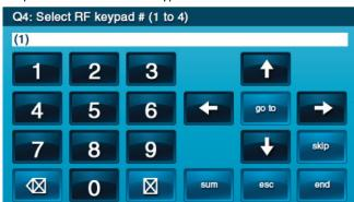
Press the → arrow or press the number 1 on the keypad toggle the setting on the first question to "used". Press the  $\downarrow$  arrow to continue configuring options.
