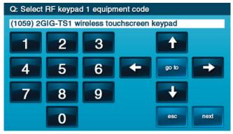
10 Learn the 2GIG-TS1 into the Control Panel. After pressing the  $\downarrow$ arrow in the previous step, the Learn button appears.
