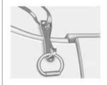
Attach the strap to the cargo tie-down in the rear of the vehicle.
