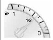
When the ignition is on, the fuel gauge indicates about how much fuel is left in the tank.
