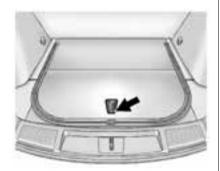
To open the cargo management system, press the rear of the handle to unlatch it and then lift the handle up.
