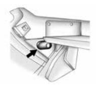
The glove box is air conditioned and can be used to store items at a lower temperature. The vehicle air conditioning must be turned on for the maximum cool air to enter the glove box. Move the slide control to allow cool air into the glove box. After opening the air flow, close the glove box door to keep the cold air from entering the vehicle.
