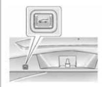
Press and release on the tailgate next to the latch to close the tailgate.
