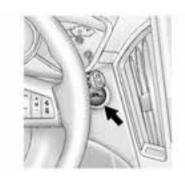
The vehicle has an electronic keyless ignition with pushbutton start.
