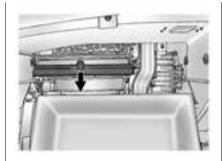
Release the two latches holding the service door. Lower the service door.
