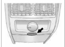
Press the button to open the storage area on the rear of the centre console. If equipped with Rear Seat Entertainment (RSE), the audio/video jacks, USB port and SD card reader may be inside. See the infotainment manual.
