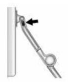
Release the prop rod from the inside cover by sliding the red clip down.
