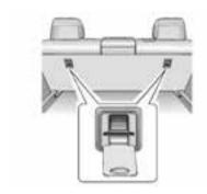
Top-tether fastening eyes are marked with so for a child seat.
