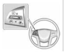
(On/Off): Press to turn the system on and off. A white indicator appears in the instrument cluster when cruise is turned on.
