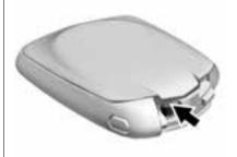
Separate the two halves of the transmitter using a flat tool inserted into the bottom centre of the transmitter. Do not use the key slot.
