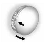
The fuel cap is behind a hinged fuel door on the passenger side of the vehicle. To open the fuel filler flap, push and release the rearward centre edge of the flap. If equipped, the fuel door is locked when the vehicle doors are locked. Press on the RKE transmitter to unlock.
