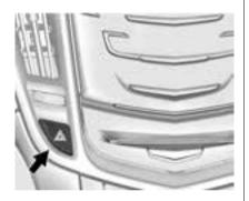
(Hazard Warning Indicators): Press this button on the instrument panel to make the front and rear indicator lamps flash on and off. This warns others that you are having trouble. Press again to turn the flashers off.
