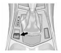
The Electric Parking Brake (EPB) switch is on the centre console. The EPB can always be activated, even if the ignition is off. To prevent draining the battery, avoid repeated cycles of the EPB when the engine is not running.
