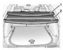
The shade can be set in two positions. It can be set in a halfway open (1) position for loading objects
