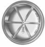
From the back side of the headlamp assembly, remove the top cap to replace the dipped beam headlamp/DRL bulb.
