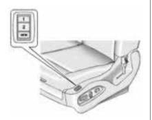
The "1," "2," and MEM buttons on the outboard side of the driver seat are used to manually save and recall the positions of the driver seat, outside mirrors, and adjustable throttle and brake pedal positions.
