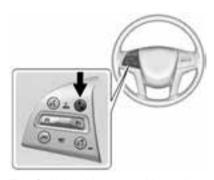
The Collision Alert control is on the steering wheel. Press on the steering wheel to set the FCA timing to far, medium, near or on some vehicles, off. The first button press shows the current setting on the DIC. Additional button presses will change this setting. The chosen setting will remain until it is changed and will affect the timing of both the Collision Alert and the Tailgating Alert features. The timing of both alerts will vary based on vehicle speed. The faster the vehicle speed,
