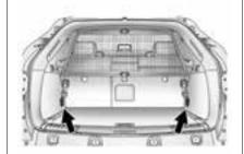
Mount the cargo net to the cargo tie-downs on the lower side panels.
