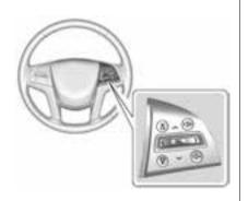
∧ or ∨ : Press the five-way control to move up or down in a list.
