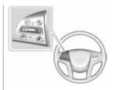
(On/Off): Press to turn the system on or off. A white cruise control indicator comes on.
