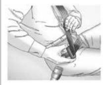
If the webbing locks in the catch plate before it reaches the buckle, tilt the catch plate flat to unlock.
