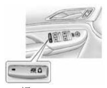
Press to activate the safety locks. The indicator light comes on when activated.
