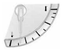
This gauge measures the temperature of the vehicle's engine.
