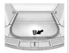
Press on the bottom of the handle assembly to unlatch it and lift up on the handle.
