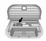
This vehicle may have a tyre sealant and compressor kit in place of a jack or spare tyre. It is located in a foam container in the rear compartment storage area. If the vehicle has a cargo cover, see Cargo Management System on page 4-5 for instructions on how to access the tyre sealant and compressor kit.
