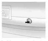
Carefully open the cover by using the small notch that conceals the rear tow eye socket.
