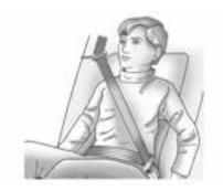
Buckle, position, and release the safety belt as described previously in this section. Make sure the shoulder portion of the belt is on the shoulder and not falling off of it. The belt should be close to, but not contacting, the neck. To remove and store the comfort guide, squeeze the belt edges together so that the safety belt can be removed from the guide. Slide the guide back into its storage pocket on the side of the seat.
