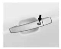
When the Remote Keyless Entry (RKE) transmitter is within 1 m (3 ft) of the driver door, pressing the lock/unlock button on that door handle will lock/unlock the doors. If the lock/unlock button is pressed again within five seconds, all passenger doors will unlock. See Remote Keyless Entry (RKE) System Operation on page 2-2.
