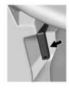
Pull the release handle with the above symbol on it. It is located below the instrument panel to the left of the steering wheel.
