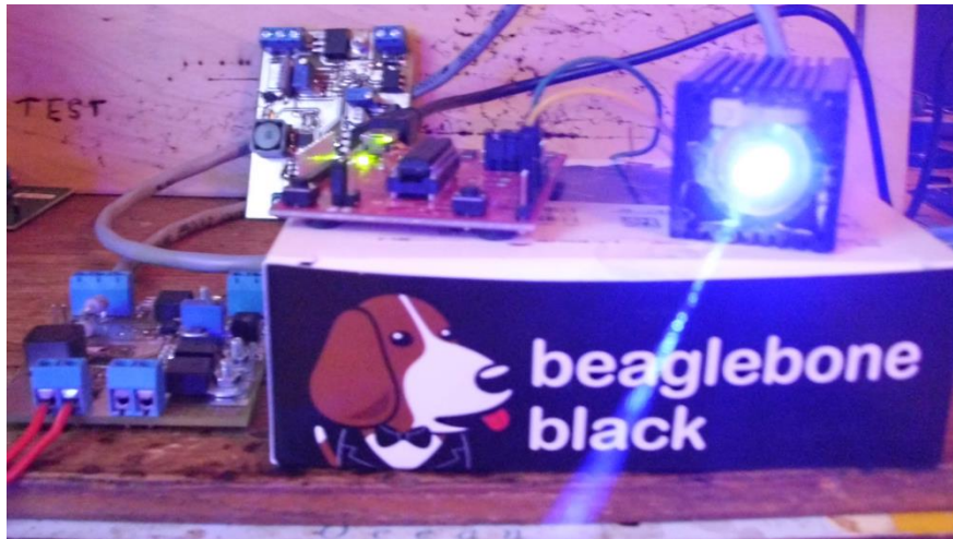
Fig. 12. MSP430 board modulating the laser
