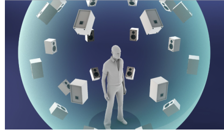
Figure 2: With ambisonics the listener can be surrounded by a large number of synthesized speakers [10].
