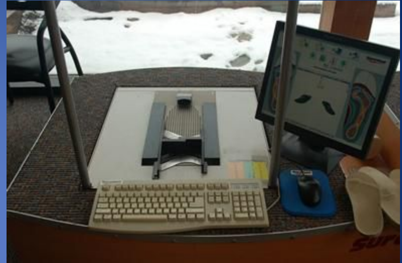
One foot at a time is scanned and 3-D modelled using this computer controlled footbed scanner.
