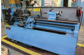
BRIDGEPORT ROMI ENGINE LATHE, MODEL 13-5, S/N 18278 210, 13" SWING, 60" CENTERS, 8" 4-JAW CHUCK, 1.5" SPINDLE BORE, (12) SPINDLE SPEEDS 50 – 2500 RPM, INCH & METRIC THREADING, TAPER ATTACHMENT
